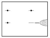
2. At each marked location, drill a ½" diameter hole.
