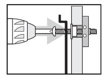
7. Once all the anchors are installed, place TV mount against installed flanges, insert bolt, and tighten against TV Mount. Ensure bolt length is at least ½" longer than the combined thickness of your TV Mount and wall.
