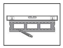
Mark anchor locations according to the TV Mount manufacturer's instructions. Ensure the mount is level when marking out anchor locations, and holes are an equal distance from the center to allow even weight distribution.
