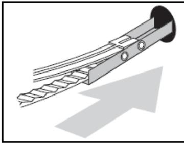
3. Fold the metal toggle against the plastic strap and insert it through the drilled hole.
