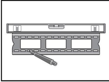
1. Mark anchor locations according to the TV Mount manufacturer's instructions. Ensure the mount is level when marking out anchor locations, and holes are an equal distance from the center to allow even weight distribution.
