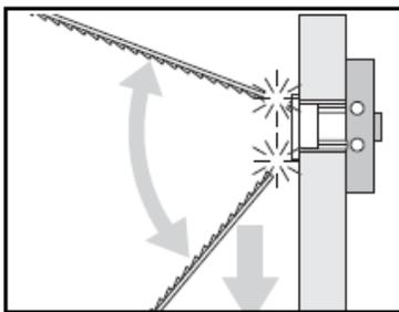
6. Gently separate straps and bend straps away from one another at the point where the strap meets the cap. Do not wiggle straps or break in same direction. Broken straps can be discarded.
