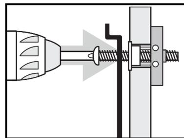
7. Once all the anchors are installed, place TV mount against installed flanges, insert bolt, and tighten against TV Mount. Ensure bolt length is at least 1/2" longer than the combined thickness of your TV Mount and wall.
