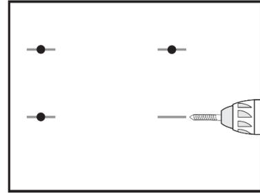
2. At each marked location, drill a 1/2" diameter hole.
